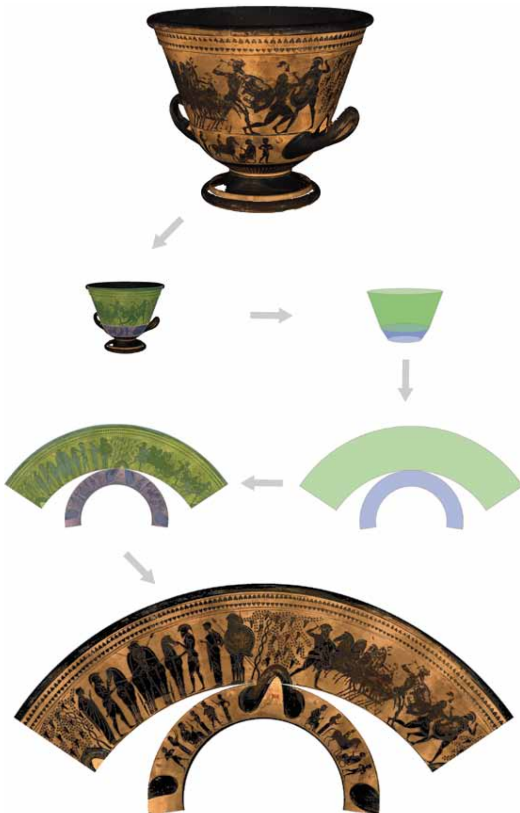
Figure 10: Schematic illustration of creating the rollout of a vessel (KHM ANSA IV 3618) that can be approximated by conical frustums and its distortion-free rollout.
